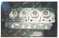
Head surfaced by machine shop note the mirror-like finish.
