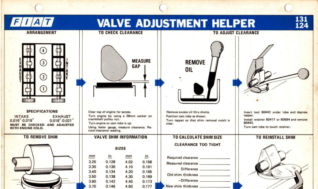
Cover area with rag. Direct air pressure at Select a shim which will give correct clearnotch to unseat shim. If shim binds, move it ance according to chart at the right. Thinner shim = more clearance Thicker shim = less clearance
