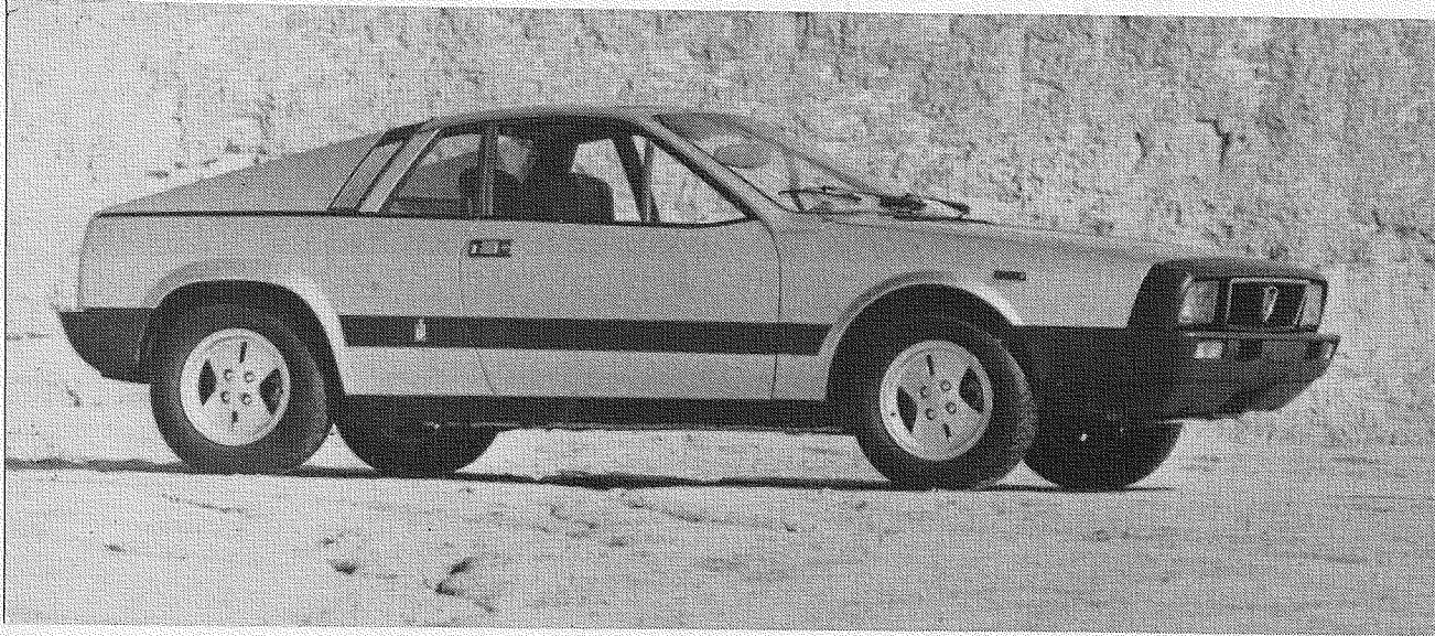
(left) Lancia Scorpion with: MonteCarlo Front End Conversion M/C Front Turn Signal/Parking Lights MonteCarlo Headlamps MonteCarlo Upper Trim Panel
